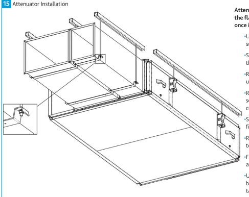
Attenuators are secured to the main unit using the flange connector on each end of the unit, once installed.
